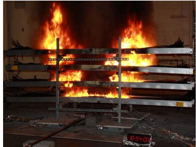
Fig. 2. Photograph of a multiple tray test involving a thermoplastic cable.
