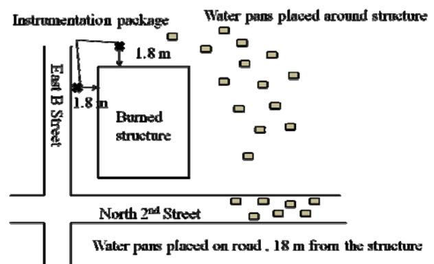
Figure 1 Location of instrumentation packages and water pans
