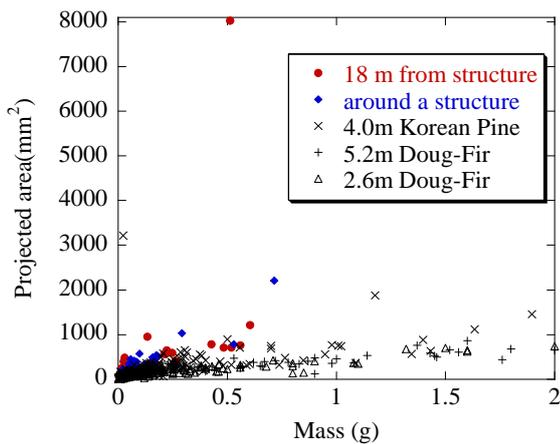
Figure 2 Mass and area of firebrands collected in this experiment, compared with firebrands generated by vegetation [4, 5].
