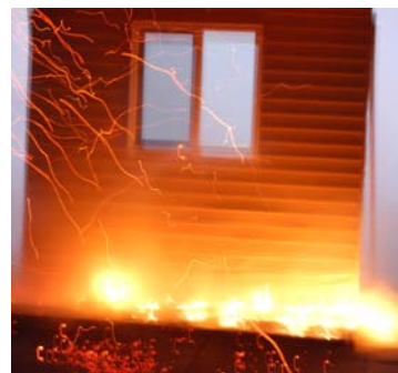
Figure 2 In the top image, firebrands have caused smoldering ignition in the mulch bed. In the bottom image, smoldering ignition has transitioned to flaming ignition and the wall assembly has ignited.
