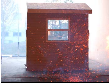
Figure 1 Picture of wall/eave assembly fitted with a vertically sliding, double hung window exposed to firebrand showers at a wind tunnel speed of 9 m/s.
