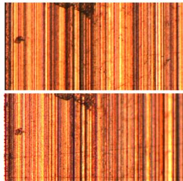
Fig. 2. Two images captured on the same area of the SRM 2460-001 bullet by the same microscope under different lighting directions. (Top) – Area aligned perpendicular to microscope optical axis, (Bottom) – The same area tilted by approximately 6°.
