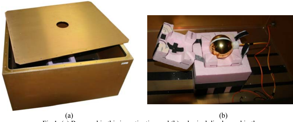
Fig 1: (a) Box used in this investigation and (b) spherical dipole used in the measurements.
