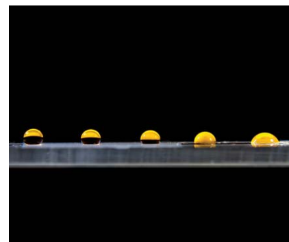
Fig. 9 The lineup: Five droplets of identical constituents and volume display gradually decreasing contact angles along the surface energy gradient. The energy gradient is created by controlling the surface roughness of a polydimethylsiloxane (PDMS) substrate through microengineering. Reproduced by permission of Weijie Cyrus Beh, Johns Hopkins University, USA.
