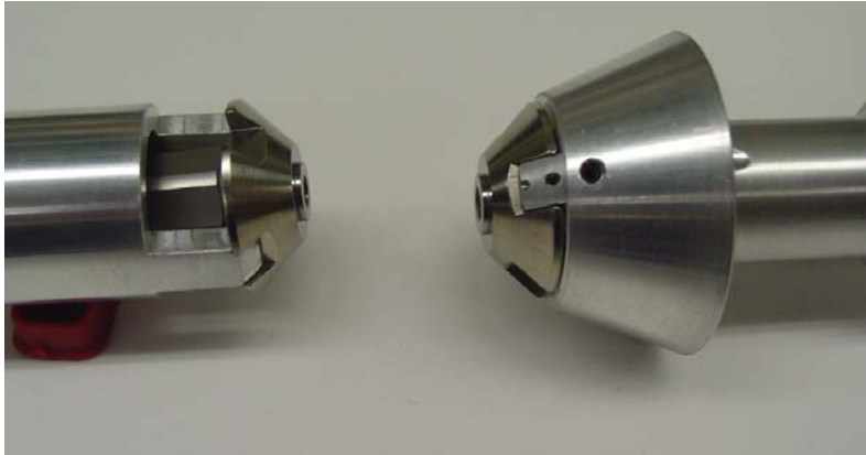
Figure 3c. Wrenches for attaching and removing mounting tables, shown with tables attached to the wrenches
