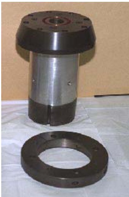
Figure 4. Inner gap assembly (left) and complete magnet assembly (right)
