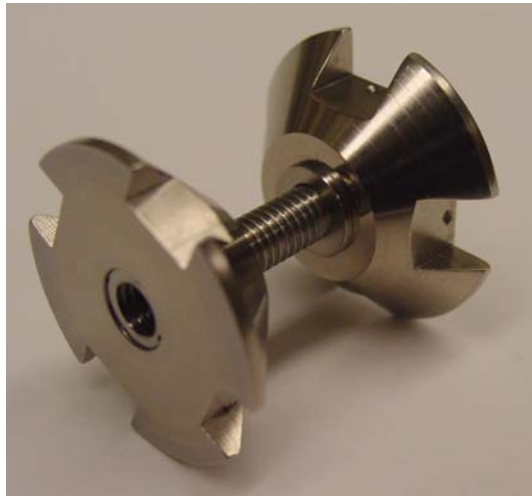
Figure 3a. Nickel-coated beryllium mounting tables for the moving element, shown with titanium threaded inserts
