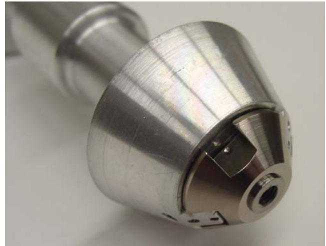
Figure 3b. Wrench for attaching and removing mounting tables, shown with table on wrench
