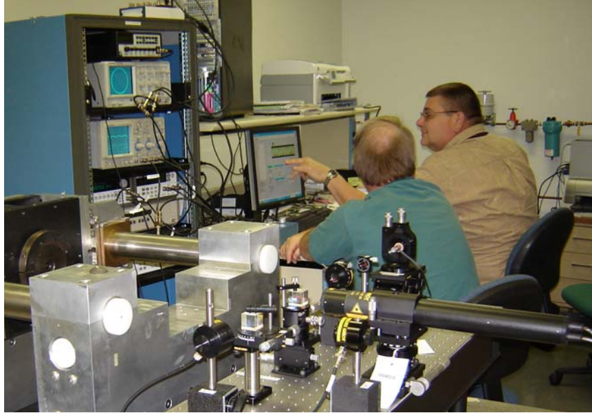
Figure 1b. SS1 with instrumentation and optical components of laser interferometer at AFMETCAL, Heath, OH
