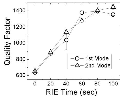
FIG. 4. Successive measurements of quality factor after plasma cleaning with 50 SCCM  $\text{O}_2$  at 50 W in an RIE. Circles represent the first mode at 13 MHz. Triangles represent the second mode at 15 MHz.
