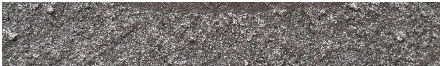
Machine off EDM Notch Remnants
