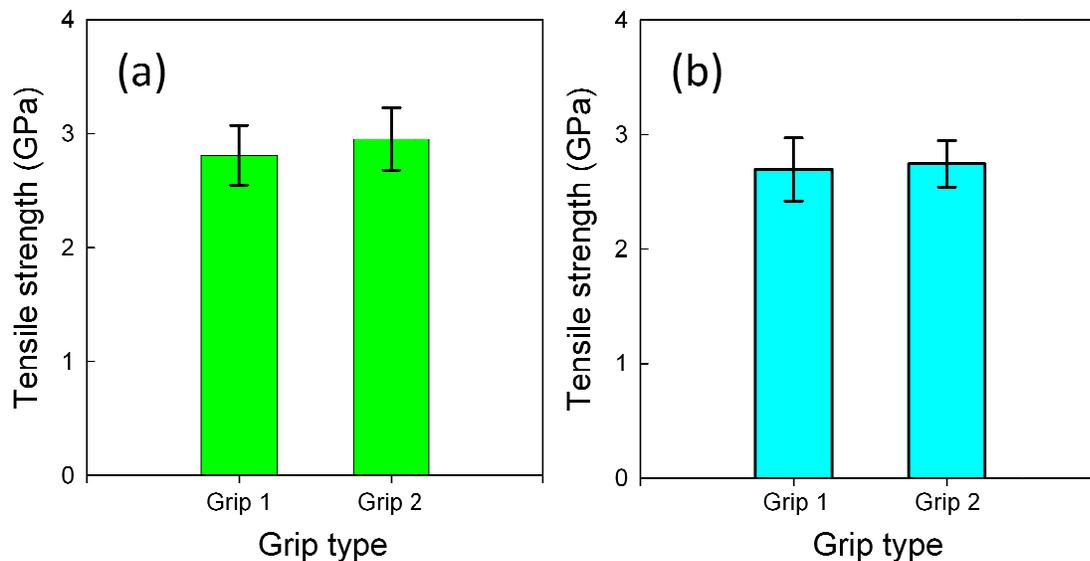
Figure 3 Single fiber tensile strength with 2 mm gauge length (a) and 60 mm gauge length (b).
