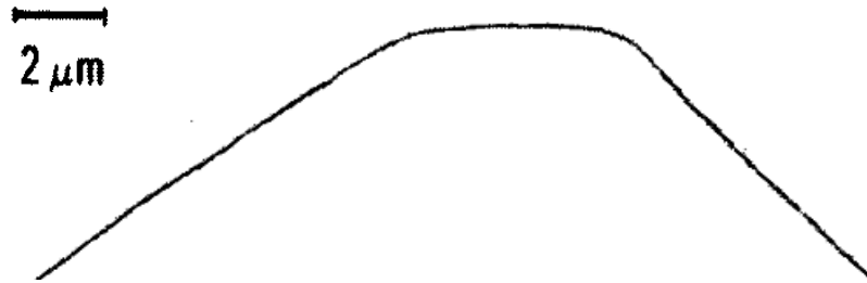
Figure 2. Razor blade profile of a stylus that was in use for many years in our laboratory. The stylus was chisel shaped with a flat about 4 \mu\text{m} across at the tip [1].
