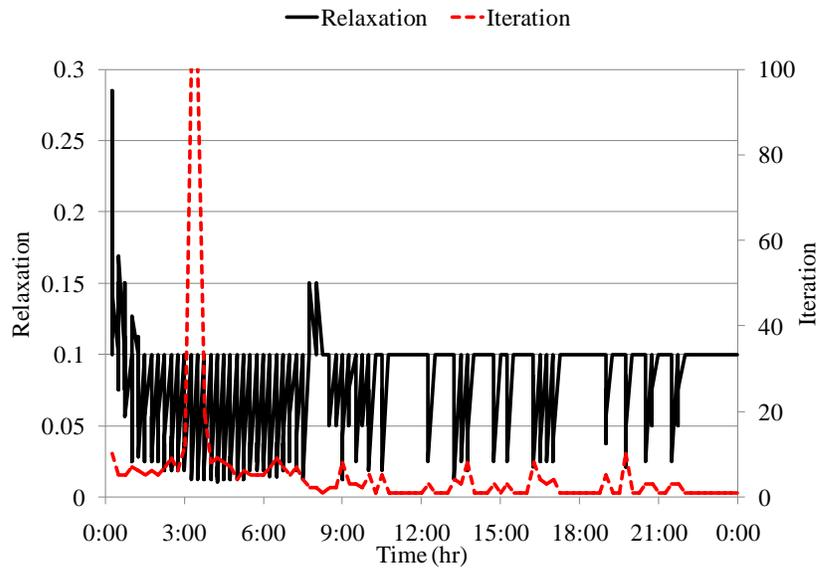
Figure 4. Adapted relaxation factors and number of iterations at each time step for the segregate solver.
