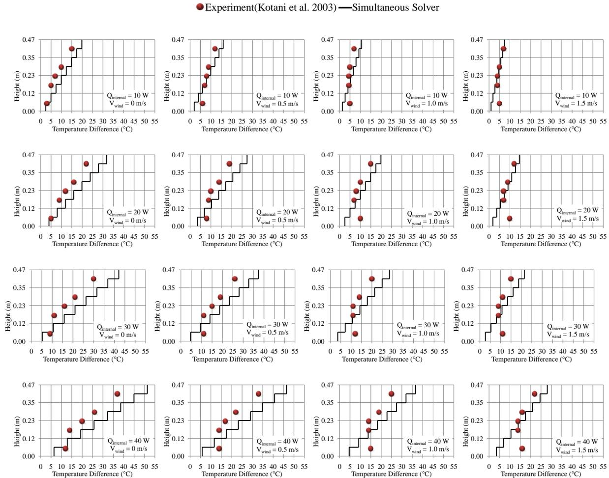
Figure 7. Comparison of predicted temperature distribution in the light well by the simultaneous solvers with measured data for different wind speeds and internal heat sources.
