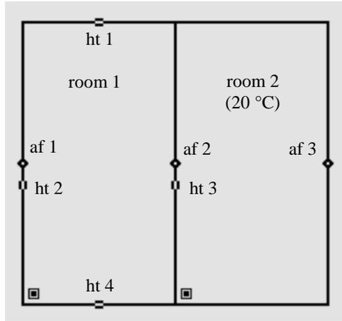
Figure 2. CONTAM97R model of the two-zone building with three airflow paths (af's) and four heat transfer paths (ht's).
