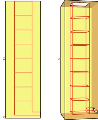
Figure 5. Airflows driven by combined wind and buoyancy effects in a light well, which is partitioned into eight sub-zones.
