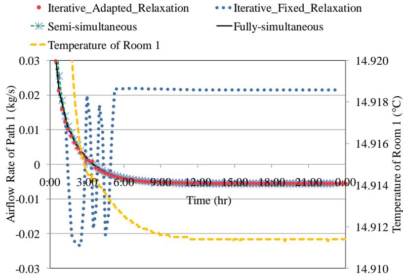
Figure 3. Comparison of predicted airflow rates through the airflow path, at 1, and temperature of room 1 by the segregate iterative solvers with adapted and fixed relaxations, and the semi-simultaneous and fully-simultaneous solvers.
