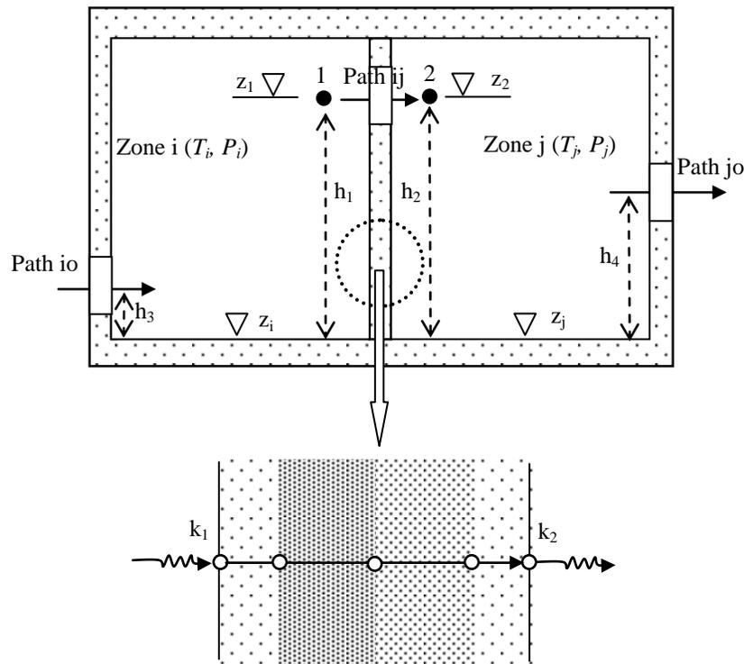
Figure 1. Schematic of airflow in a two-zone building and enlarged heat transfer at the surface and through an internal wall assembly.
