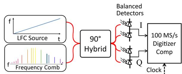
Fig. 1. (Color online) Basic schematic of the LFC source characterization against the fiber-laser frequency comb using optical IQ demodulation.
