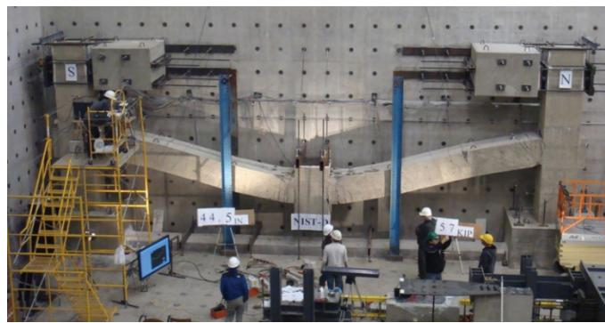
**Fig. 13.** Photograph of concrete SMF assembly in post-ultimate-load position
