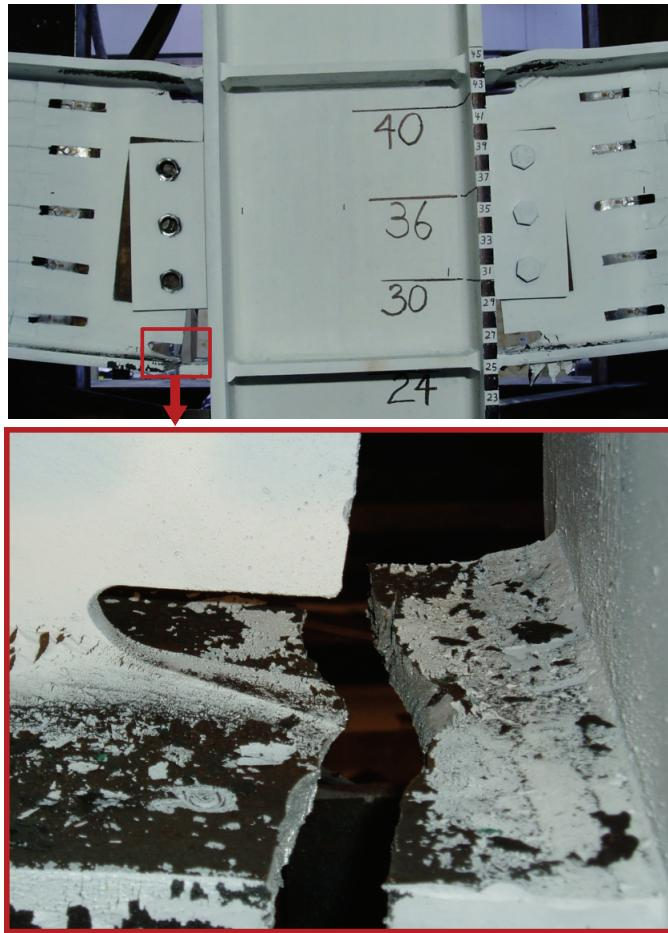
**Fig. 4.** Failure mode of steel IMF assembly
