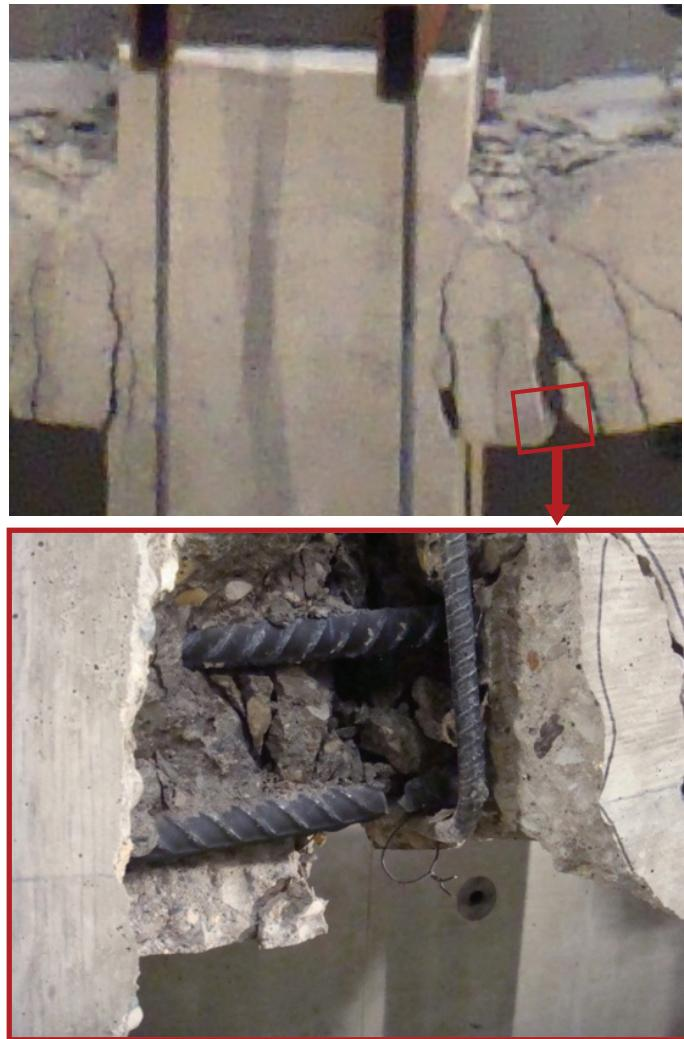
**Fig. 19.** Failure mode of concrete SMF assembly
