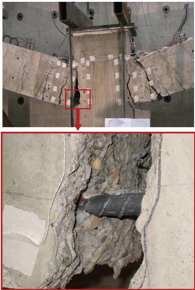
**Fig. 15.** Failure mode of concrete IMF assembly
