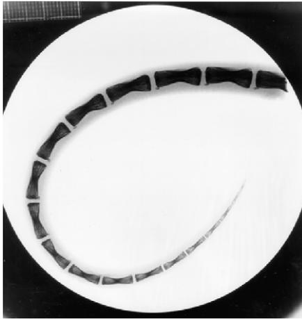
Fig. 7. Image of mouse tail obtained by using Ag LHXs driven by high contrast laser pulses. The mesh scales as 1 cm.
