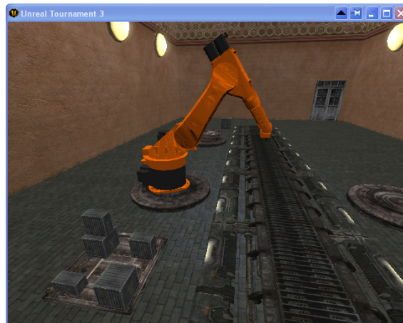
Figure 4: View of the USARSim physics-based simulation of a mixed-pallet under construction.
