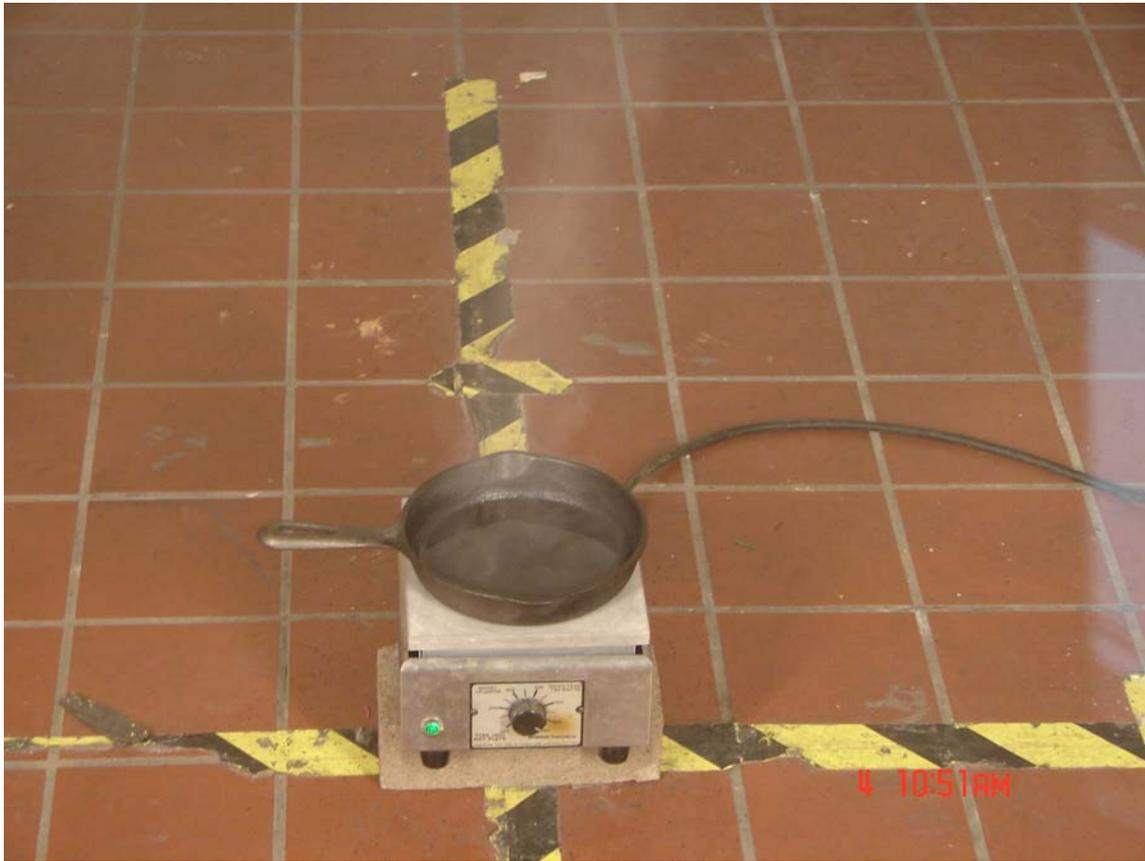
**Figure 2 Vegetable oil heated in a 14 cm diameter skillet on a hotplate**
