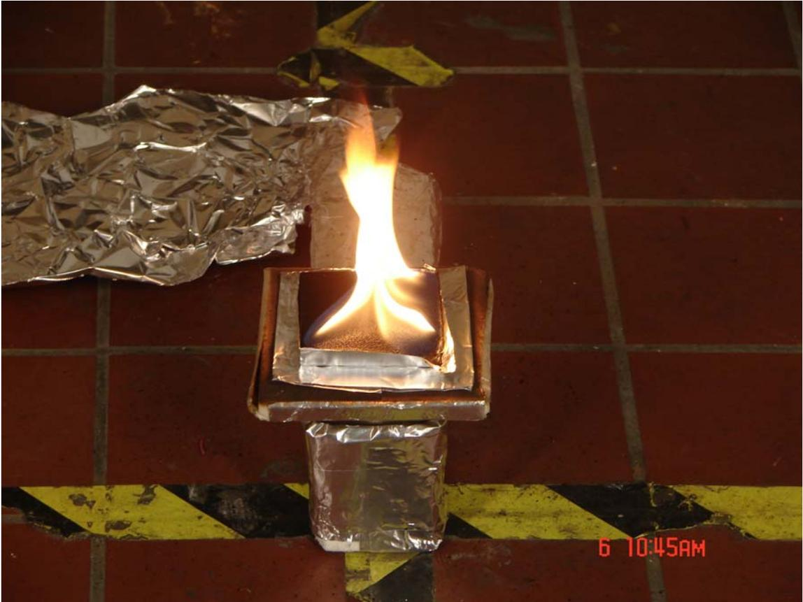
**Figure 3 Flaming PMMA on the load cell**
