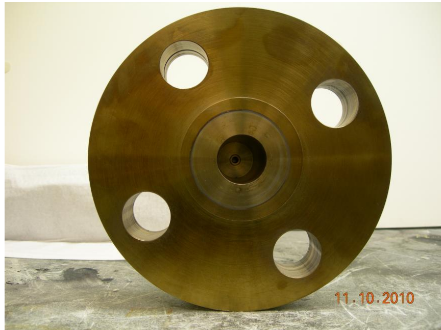
Figure 8. Postmortem photograph of Vessel #5 (vessel body with O-ring removed) after exposure at 427 °C for 9 h.
