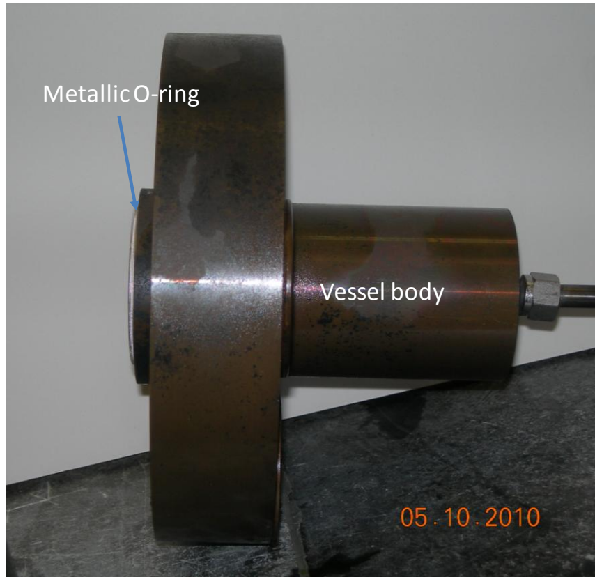
Figure 3. Postmortem photographs showing silver from the metallic O-ring deposited on the O-ring groove and the O-ring bonded to the tested vessel (Vessel #1) body.
