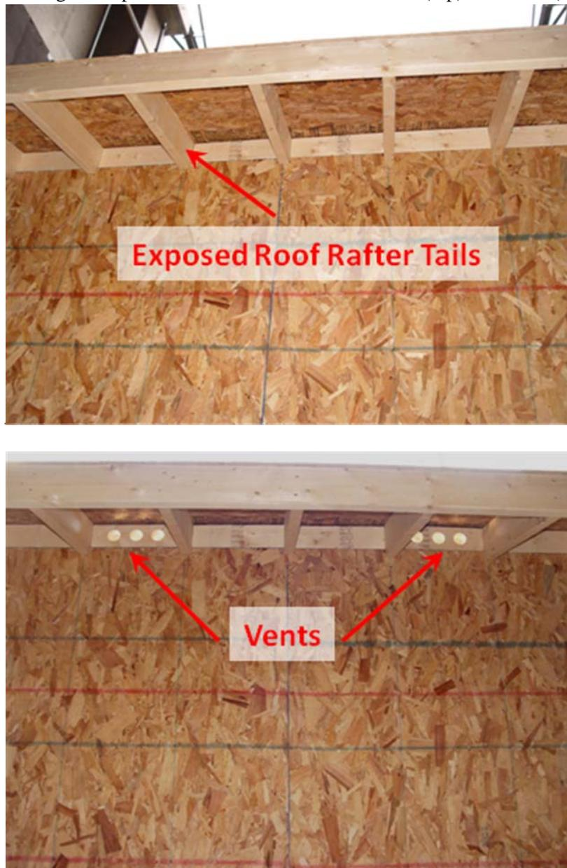
Figure 7 displays a typical experiment showing a wall fitted with an eave exposed to firebrand showers from the NIST Dragon inside the FRWTF. For the experiments that used no vent opening,
