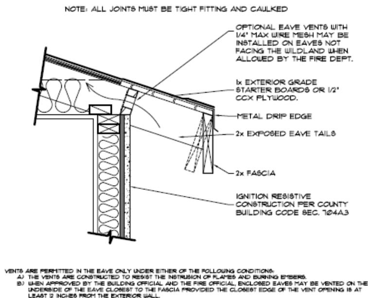
Figure 5 displays common open eave constructions used in California. The construction found in
