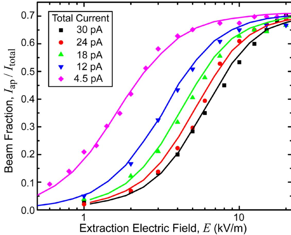
FIG 6. Fraction of beam current passing a 20  $\mu\text{m}$  aperture vs extraction electric field for various beam currents. Symbols are experimental data and solid lines are Monte Carlo simulations. Uncertainties of the measured data are  $\pm 7\%$ .
