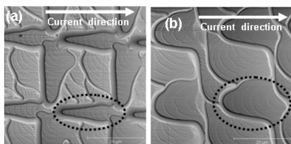
FIG.4: AFM images showing the evolution of the step-terrace patterns originating from the trenches as shown by the dashed circles. The images are taken at two different times during the annealing.
