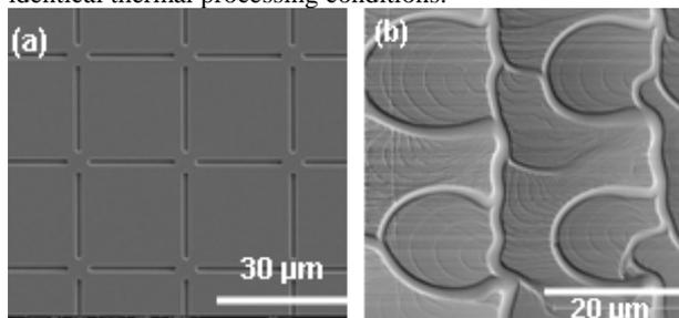
FIG. 2: (a) Scanning electron micrograph of the  $25\mu\text{m}$  square pattern. (b) Corresponding AFM image after  $1050^\circ\text{C}$  anneal of 18 hours. The current direction is from left to right.
