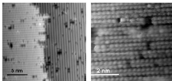
FIG.5: High resolution image of the samples acquired using scanning tunneling microscope. Figures show long range atomic scale ordering with dimmer row reconstruction.
