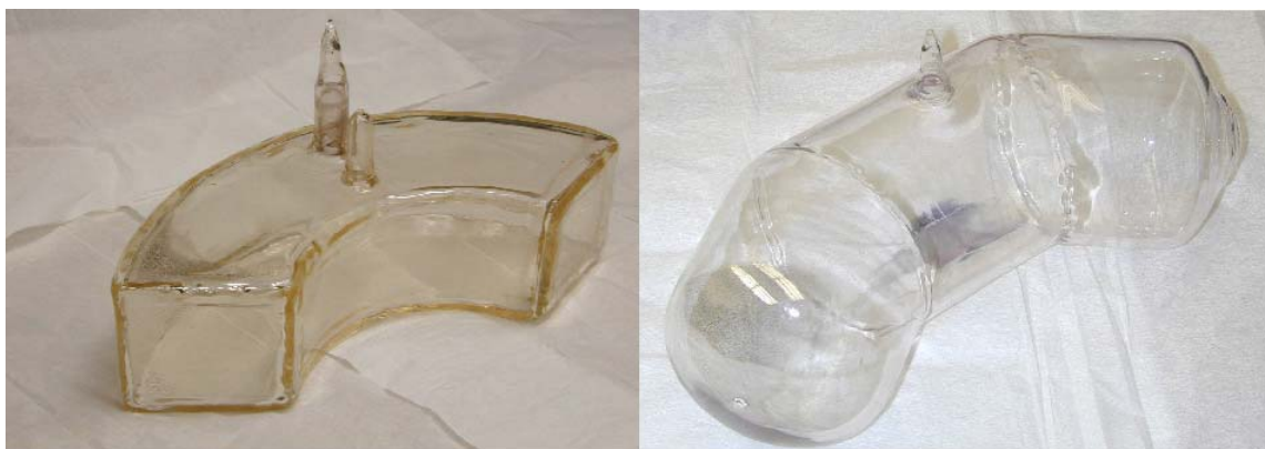
Figure 9. One of each type of fused quartz cells for wide-angle analysis cells: welded cell Rainbow (left) and cell Jersey (right) made from three connected sections of slightly resized tubing.
