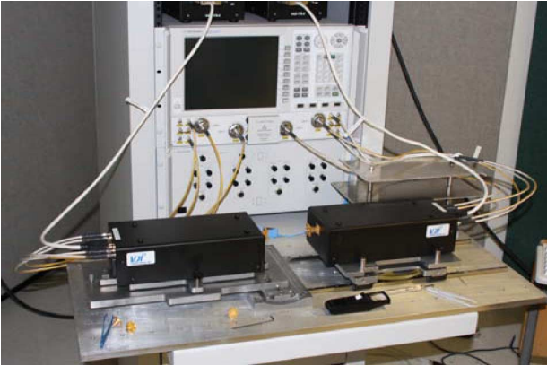
Fig. 1. The rail system we built to constrain the movement of the extension heads and cables.
