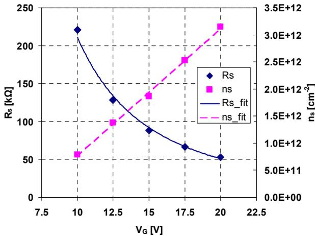
Fig. 5. Sheet resistance and inversion sheet charge density measured at different gate voltages.
