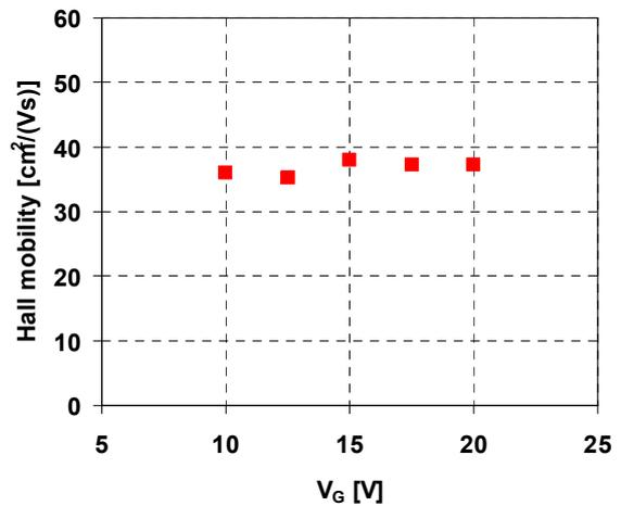
Fig. 6. Hall mobility calculated from  $R_s$  and  $n_s$  as a function of gate voltage.
