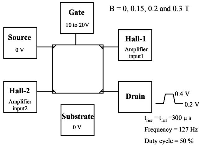
Fig. 2. The 4H-SiC Van der Pauw structure measured, which has an active gate area of 150  $\mu\text{m} \times 150 \mu\text{m}$ . The setup shown here is for the inversion sheet charge density ( $n_s$ ) measurement.
