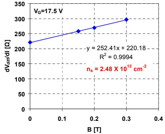
Fig. 4. Inversion sheet charge density ( $n_s$ ) extraction at  $V_G=17.5$  V.
