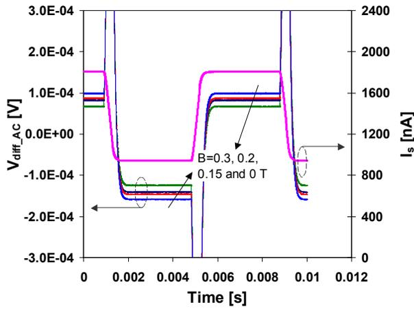
Fig. 3. Source current and differential voltage corresponding to the drain voltage modulation. Four magnetic fields are used. As B increases,  $dV_{diff}$  gets larger.
