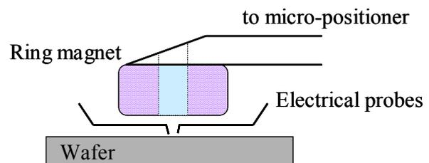
Fig. 1. Wafer-level Hall measurement setup. The magnetic field is provided by a permanent ring magnet. The distance from the wafer is controlled by a micro-positioner.
