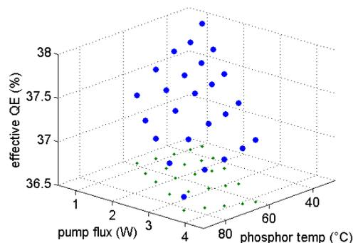
**Figure 3.** Effective QE for LED2 as a function of phosphor temperature and initial pump flux (large blue dots) and its projection in the horizontal plane (small green dots).
