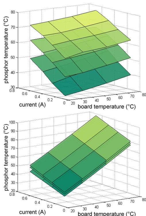
**Figure 2.** Phosphor temperature of LED1 (top) and LED3 (bottom) as a function of the forward current and board temperature for 25 °C, 40 °C, and 55 °C ambient sphere temperatures.
