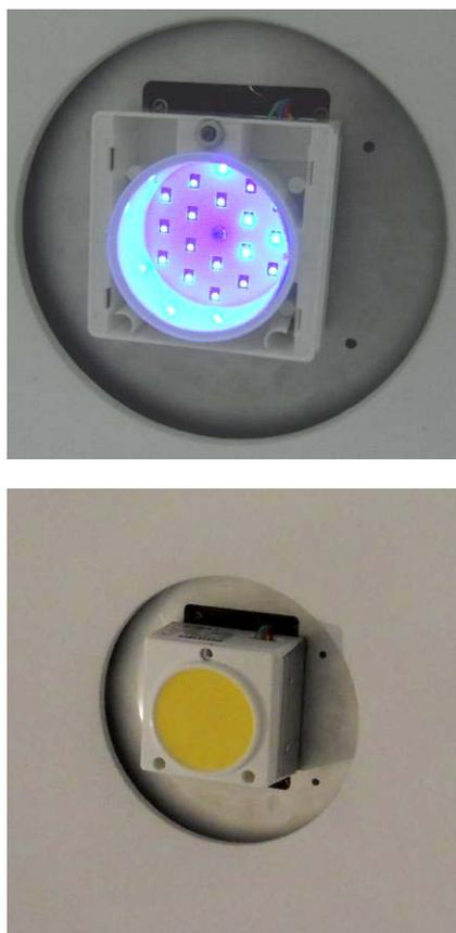
**Figure 1.** Remote phosphor type LED mounted on the sphere surface without (top) and with (bottom) its remote phosphor plate.
