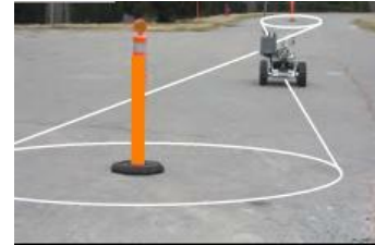
Figure 2: Paved Surface Terrain-for Sustained Speed and Towing Test Methods
