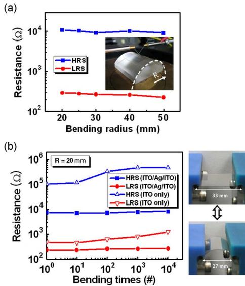
**Fig. 5.** (a) HRS and LRS data from a flexible ZnO unipolar resistive switching device as a function of the bending radius. (b) Data for the HRS and LRS following multiple flexes at  $R = 20$  mm. Reprinted with permission from [64] © 2009, American Institute of Physics.
