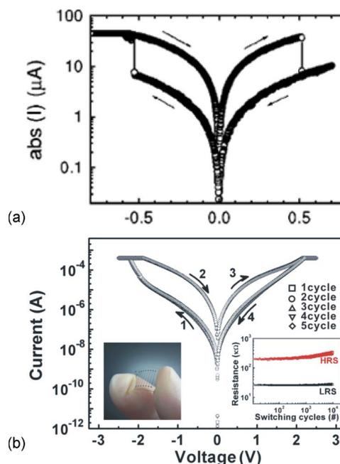
**Fig. 2.** Bipolar switching consistent with memristor behavior is evident for (a) an inflexible  $\text{SrZrO}$  device. Reprinted with permission from [27] © 2000, American Institute of Physics. (b) Similar bipolar switching is also evident for flexible  $\text{Al/TiO}_2/\text{Al}$  devices formed on polyethersulfone. Reprinted with permission from [46] © 2010, IOP Publishing, Ltd.
