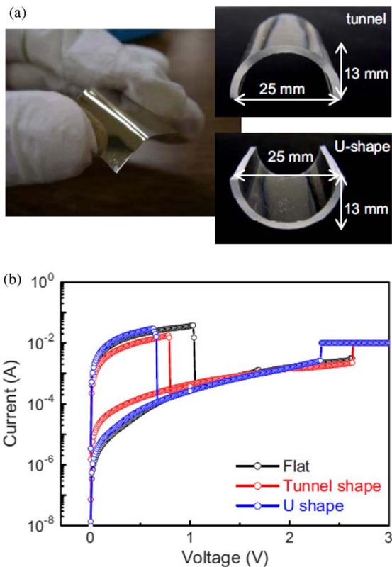
**Fig. 3.** (a) Photograph of a flexible ZnO unipolar resistive switching device being flexed. (b) Typical switching characteristics for the device shown in (a). Reprinted with permission from [45] © 2009, American Institute of Physics.
