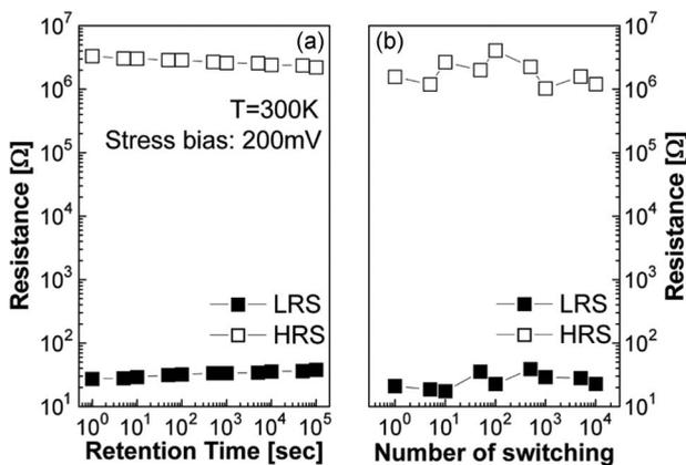
**Fig. 6.** (a) Data retention characteristics for a flexible ZnO unipolar resistive switching device over time. (b) Endurance tests. Reprinted with permission from [63].
