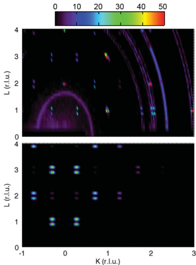
FIG. 2. (Color online) (a) Pattern of elastic intensity at  $T = 1.5$  K measured on BT9 in the  $(0KL)$  zone. The circles at high and low  $q$  arise from the Al powder and  $^4\text{He}$ , respectively. (b) Calculated scattering pattern for long-range magnetic order using the spin-density-wave magnetic configuration, which is domain-averaged as described in the text.
