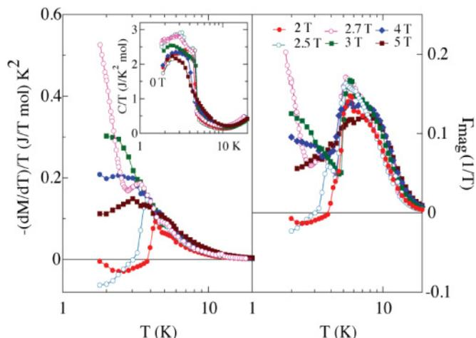
FIG. 4. (Color online) (a) Differential magnetic susceptibility at different fields as a function of temperature.  $C(T)/T$  at different fields as a function of temperature are shown in the inset. (b) Variation of Gruneisen ratio parameter at different fields.
