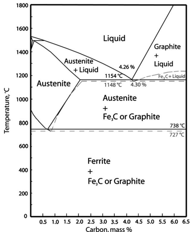
Fig. 2 – The stable iron–carbon phase diagram with the metastable Fe– $\text{Fe}_3\text{C}$  system in gray dashed lines.
