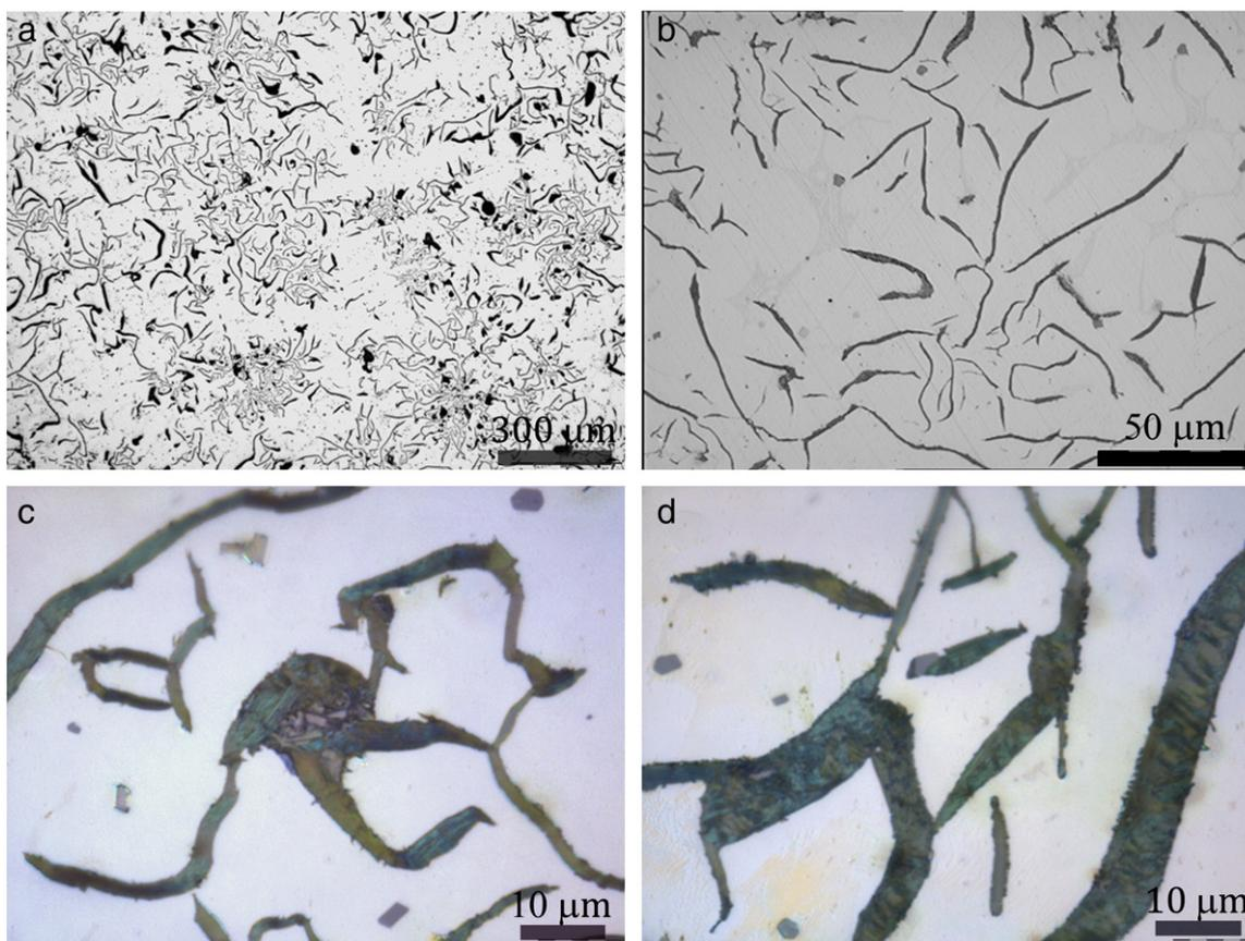
**Fig. 3** – Graphite flake morphologies typical of the skin on the U.S. Capitol dome: (a) as-polished, showing mostly type B rosette graphite structures, (b) as polished showing mostly type A graphite flakes, (c) internal structure of graphite with cross-polarized light, and (d) internal structure of graphite flake under cross-polarized light. (For interpretation of the references to color in this figure legend, the reader is referred to the web version of this article.)
