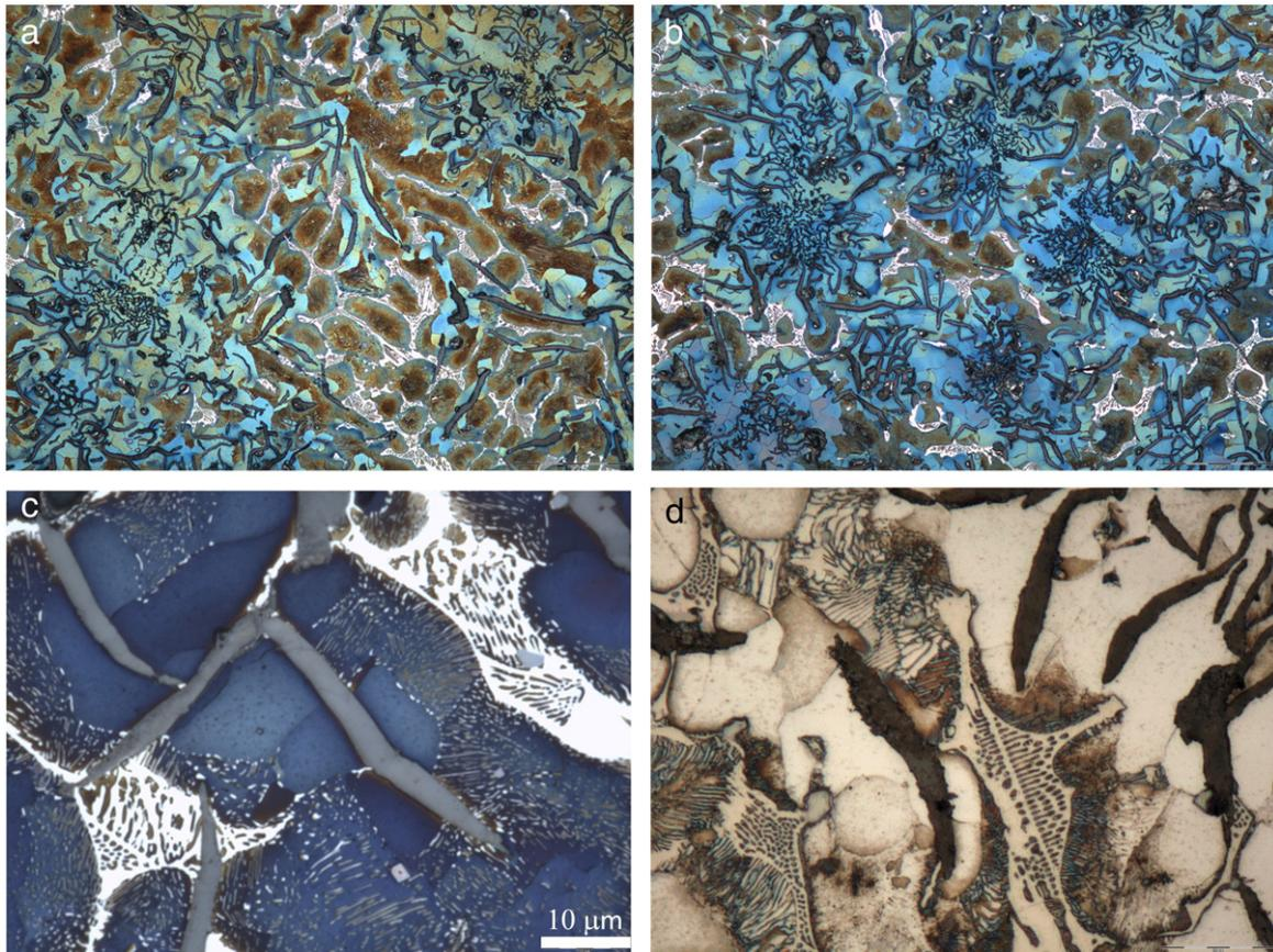
**Fig. 4** – Microstructure of the skin castings shown with Beraha's etch in a–c, with pearlitic regions in brown, steadite in white, ferritic regions in blue, and graphite in black. In d, a similar region to c has been etched with Klemm's etch, which reduces the contrast between steadite and ferrite. (For interpretation of the references to color in this figure legend, the reader is referred to the web version of this article.)
