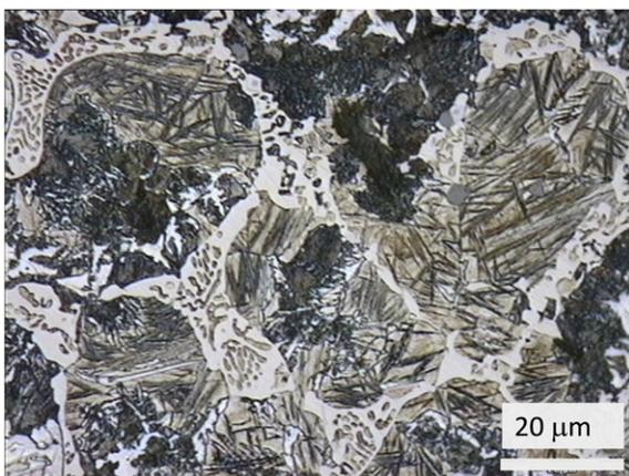
**Fig. 5** – Optical micrograph of martensite formed during a weld cooling cycle, obtained with Beraha's etch.
