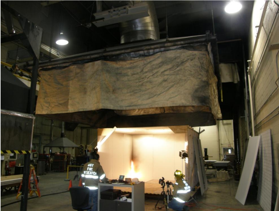
Figure 6. Fire pattern compartment located under 10 m hood in the NIST Large Fire Laboratory. In this case a corner fire pattern was being generated.
