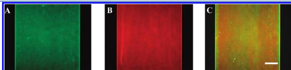
**Figure 3.** Images of fluorescently labeled components of the hCAM. (A) PAH–FITC and (B) FN–ROX deposited on four layers of polyelectrolytes ((PAH/PSS)<sub>2</sub>). (C) PAH–FITC deposited on FN–ROX and both on (PAH/PSS)<sub>2</sub>. The color in (C) denotes the overlapping of the labeled PAH and FN throughout the surface. Scale bar 200  $\mu\text{m}$ .
