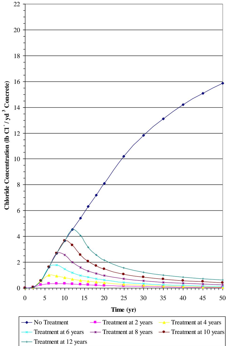
**FIGURE 2 Chloride concentrations at the level of reinforcing steel in decks with SIPMFs and a 3.0-in. (76.2 mm) OCD for 1.0-in. (25.4 mm) scarification and 2.0-in. (50.8 mm) overlay treatments (depth of reinforcing steel is 3.0 in. (76.2 mm) for no-treatment case and 4.0 in. (101.6 mm) for treatment cases).**
