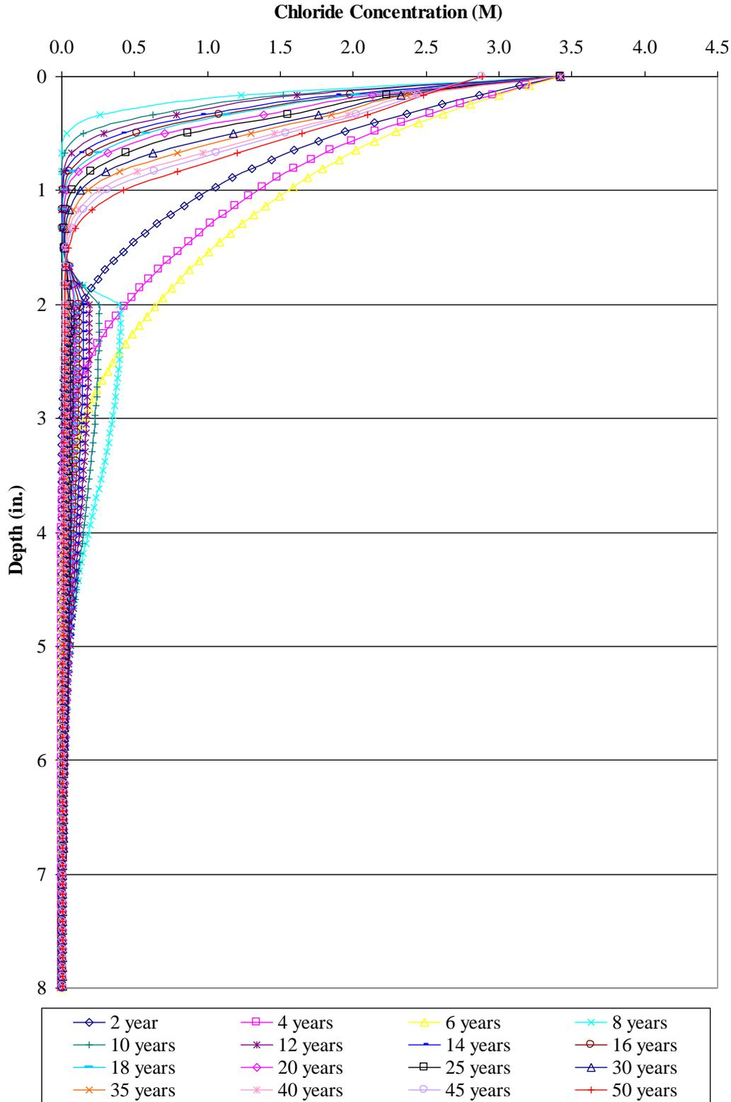
**FIGURE 1 Chloride concentrations of decks with SIPMFs and a 3.0-in. (76.2 mm) OCD and a 1.0-in. (25.4 mm) scarification and 2.0-in. (50.8 mm) overlay treatment applied at 6 years.**
