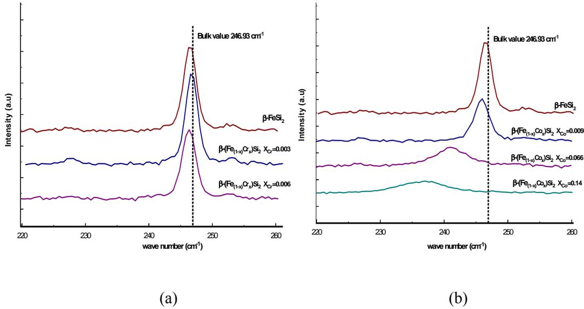
**Figure 1:** The  $A_{1g}$  Raman peak for the (a) Cr doped samples and (b) Co doped samples are shown for comparison. The Raman spectra for the nominally undoped sample is included in both (a) and (b), and the vertical line at  $246.93 \text{ cm}^{-1}$  represents the peak position for fully relaxed single crystalline  $\beta\text{-FeSi}_2$ .
