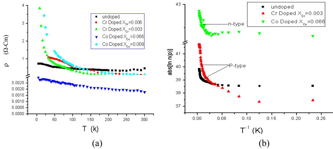
**Figure 2:** Temperature dependence of (a) resistivity (b) Carrier concentration for undoped, Cr doped and the Co doped samples is shown for comparison.
