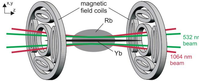
FIG. 1. (Color online) Sketch of the trapping geometry for  $^{174}\text{Yb}$  and  $^{87}\text{Rb}$  showing the trap lasers and magnetic field coils (not to scale). Coordinate axes  $x, y, z$  are indicated.
