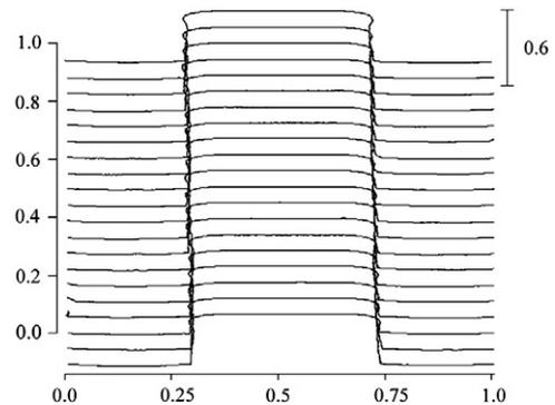
Fig. 4. Grating profile measured by AFM with all scales in micrometers. Line profiles show a clear presence of an overhang on the top of the grating.
