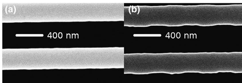
Fig. 1. Scanning electron microscope images from above (a) unperturbed and (b) perturbed line grating.
