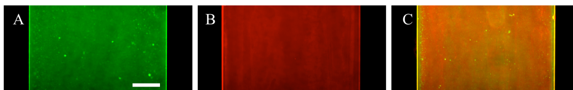
Figure 2. Micrographs of fluorescently labeled components of hCAM. A) PAH-FITC deposited on top of (PAH/PSS)_2 . B) Fibronectin-ROX deposited onto (PAH/PSS)_2 . C) PAH-FITC deposited onto fibronectin-ROX, and all onto (PAH/PSS)_2 . Scale bar: 200 \mu\text{m} .
