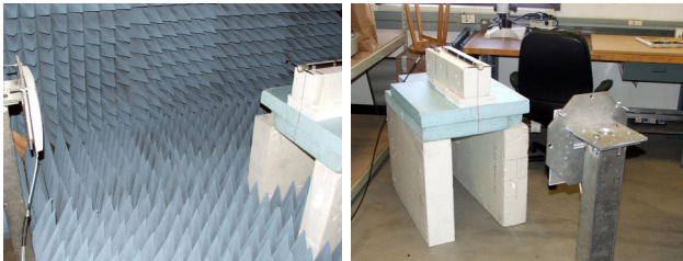
Figure 5 – The semi-anechoic chamber (left) and storage room (right) test environments. The LP reader antenna is shown in each on its steel mounting structure, boresight to the dipole target.
