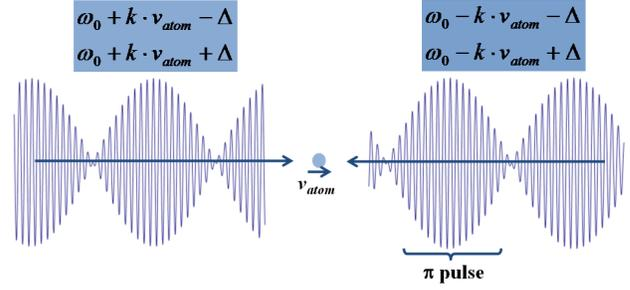
Fig. 2. The bichromatic cooling scheme.
