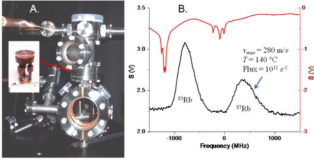
Fig. 3. A. A picture of our bichromatic cooling apparatus. The atomic beam collimator is shown in the inset. B. Velocity distributions measured with our apparatus (black) and a saturated absorption signal used for calibration (red).
