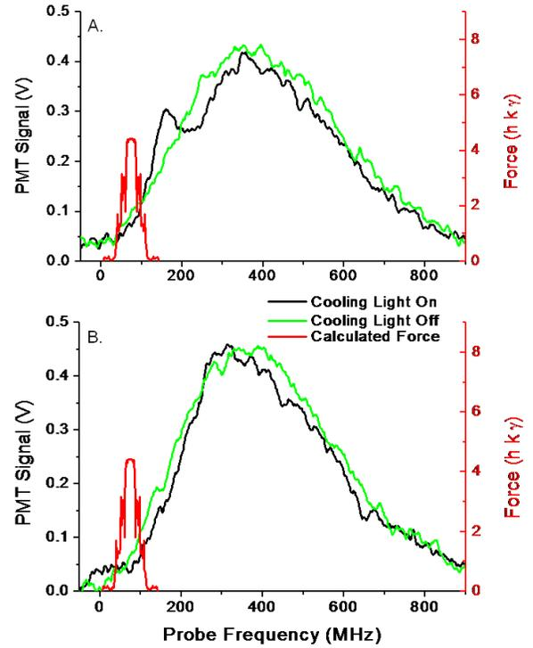
Fig. 4. Measured velocity distributions with and without the bichromatic cooling beams on (left axis). The expected force profile for our experimental parameters is also shown (right axis). A.) Measured distributions with the beat phase for the bichromatic cooling beams set to speed up the atoms. B.) Measured distributions with the beat phase set to produce slowing. Note that some of the atoms have negative velocity in the detection region.
