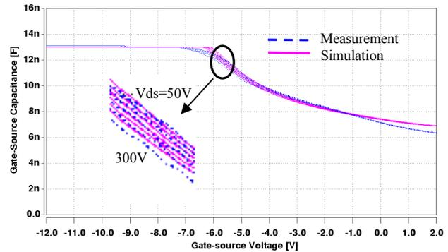
**Fig. 8** Gate-Source capacitance versus gate-source voltage of the 650 V, 60 A (0.57 cm<sup>2</sup>) CoolMOS<sup>TM</sup> transistor at 25 °C for drain-source voltage at 50 V, 100 V, 150 V, 200 V, 250 V, and 300 V with zoomed-in plot.
