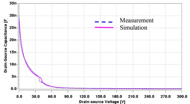
**Fig. 9** Drain-Source capacitance versus drain-source voltage of the 650 V, 60 A (0.57 cm<sup>2</sup>) CoolMOS<sup>TM</sup> transistor at 25 °C.
