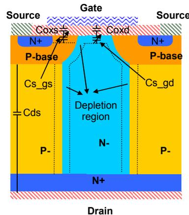
**Fig. 1** Cross-section of the CoolMOS<sup>TM</sup> transistor with inter-electrode capacitances model topology superimposed.
