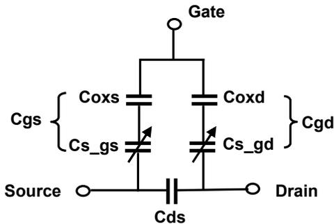
Fig. 2 The simplified equivalent circuit of the CoolMOS<sup>TM</sup> transistor in the nonconducting state.
