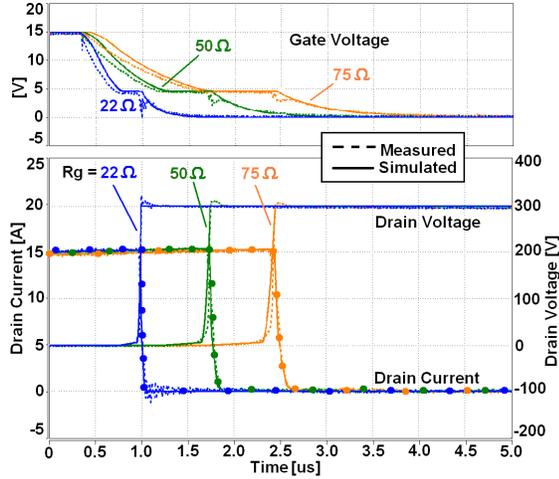
Fig. 12 Simulated (solid) and measured (dashed) inductive load switching waveforms of gate voltage (top); and drain current at 15 A (with dots) and drain voltage at 300 V for  $R_g = 22 \Omega$ ,  $50 \Omega$ , and  $75 \Omega$  at  $25^\circ\text{C}$ .
