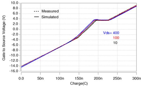
**Fig. 10** Gate charge results of the 650 V, 60 A (0.57 cm<sup>2</sup>) CoolMOS<sup>TM</sup> transistor at 25 °C.
