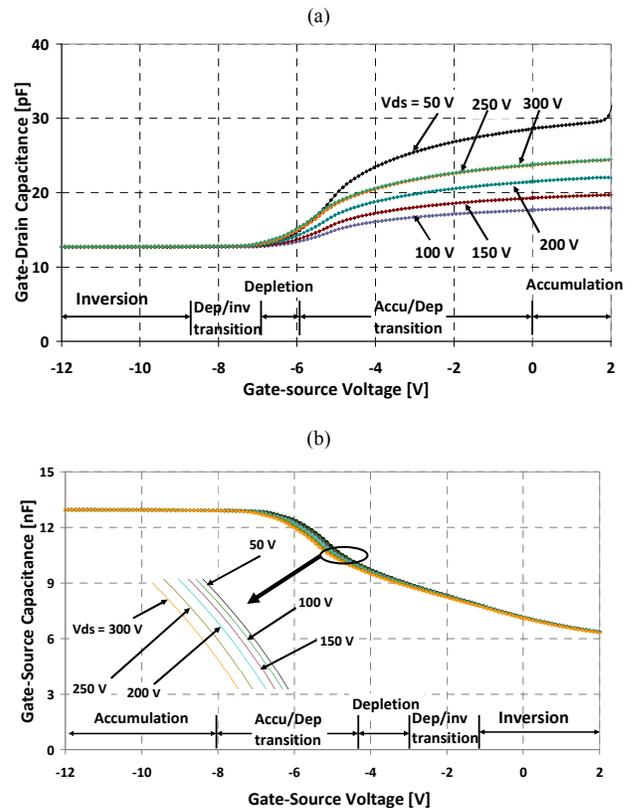
Fig. 3 (a) Transition from the region of accumulation to depletion and then inversion of  $C_{gd}$  with decreasing  $V_{gs}$ . Notice that the curves overlap for  $V_{ds} = 250$  V and 300 V; (b) transition from the region of accumulation to depletion and then inversion of  $C_{gs}$  with increasing  $V_{gs}$ .
