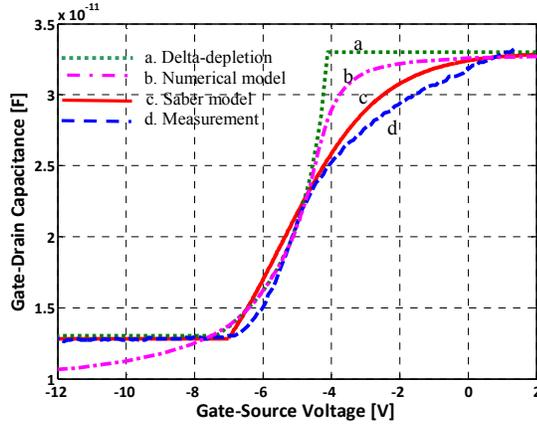
**Fig. 4** Comparison of (a) the delta-depletion model (dotted), (b) the numerical model (dash-dot), (c) the simplified model simulation (solid), and (d) the measured (dashed)  $C_{gd}$  versus  $V_{gs}$  curves of a 650 V, 60 A CoolMOS™ for drain-source voltage at 50 V.
