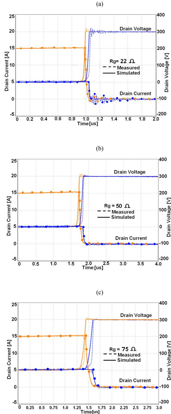
**Fig. 11** Simulated (solid) and measured (dashed) inductive switching turn-off waveforms of drain current (dotted) and drain voltage at 25 °C for (a)  $R_g = 22 \Omega$ ; (b)  $R_g = 50 \Omega$ ; and (c)  $R_g = 75 \Omega$ .
