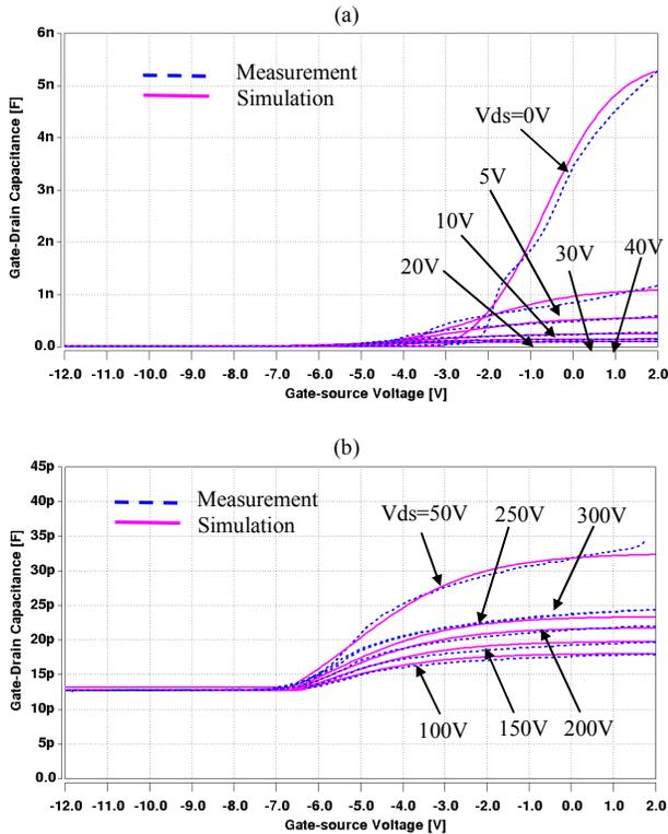
**Fig. 6** Gate-Drain capacitance versus gate-source voltage of the 650 V, 60 A (0.57 cm<sup>2</sup>) CoolMOS<sup>TM</sup> at 25 °C for drain-source voltage (a) at 0 V, 5 V, 10 V, 20 V, 30 V, and 40 V; and (b) at 50 V, 100 V, 150 V, 200 V, 250 V, and 300 V.
