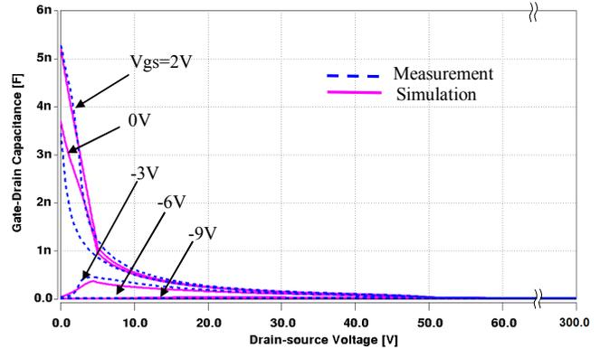
**Fig. 7** Gate-Drain capacitance versus drain-source voltage of the 650 V, 60 A (0.57 cm<sup>2</sup>) CoolMOS<sup>TM</sup> transistor at 25 °C for drain-source voltage sweeping from 0 V to 300 V by condensing  $V_{ds}$  between 60 V to 300 V.
