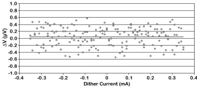
Fig. 6. Measured output voltage deviation from the expected quantized dc voltage versus dither current for a 10 V PJVS with all 32 subarrays active. These particular data demonstrate a perfectly flat “operating margin” of 0.7 mA (for the device in Fig. 3(a) having  $I_c \approx 4.8$  mA). The dither bias current flows simultaneously through all cells.
