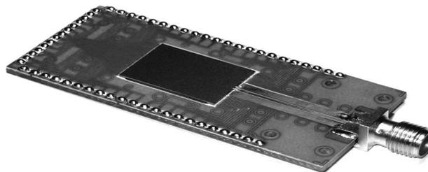
Fig. 4. Photograph of a newly developed flip-chip-on-flex cryopackage for the 10 V PJVS devices. The 330  $\mu$ m center-to-center finger spacing of these new cryopackages is half that of their predecessors due to the large number of wiring connections required (and the fact that the 12 mm-by-17 mm 10 V circuits have room for pads on only two sides).
