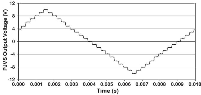
Fig. 1. Digital oscilloscope measurement of a 10 V (zero-to-peak) 100 Hz triangle wave generated by the 10 V PJVS system. This 10 V circuit design consists of 32 equally sized subarrays, giving a “digital” resolution around 400 mV. We are also developing a new “high-resolution” 10 V PJVS chip, and these more versatile devices will have a least significant bit of approximately 200  $\mu\text{V}$ .
