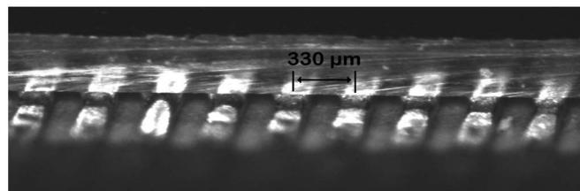
Fig. 5. Magnified view of the InSn solder bonds between (top) a 10 V PJVS silicon chip and (bottom) the copper traces on the “flex” microwave dielectric base layer. The recently reengineered chip-bonding machine precisely controls the thickness of the solder in the gap (approximately 50  $\mu$ m on this cryopackage). (*Note: The mirror finish of the diced chip edge shows the reflection of the copper fingers below.*)
