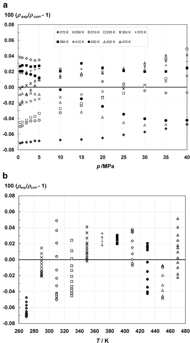
**Figure 4.** (a) Deviations of density data of compressed-liquid JP-8 3773 from the correlation (eq 4), as a function of the (a) pressure and (b) temperature.
