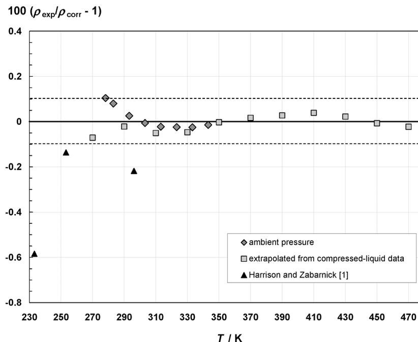
**Figure 3.** Deviations of measured and extrapolated ambient pressure density data of JP-8 3773 from the correlation (eq 3). Also shown are deviations of the data by Harrison and Zabarnick.<sup>1</sup>
