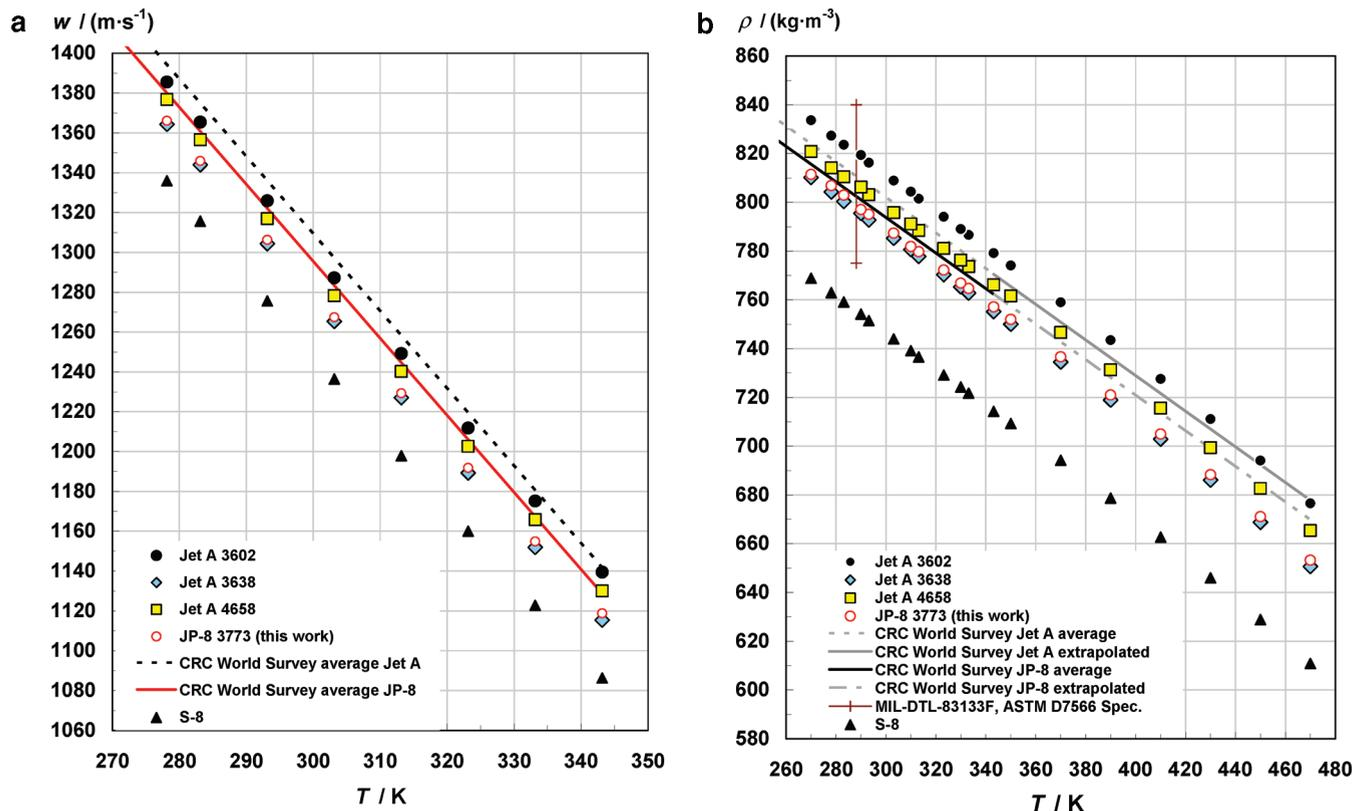
Figure 1. (a) Measured speed of sound data and (b) measured and extrapolated density data of JP-8 3773 compared to three other Jet A fuels reported previously in ref 13 and the correlations for the speed of sound and density, respectively, of average Jet A and JP-8 from the CRC World Survey<sup>19</sup> as a function of the temperature at ambient pressure.
