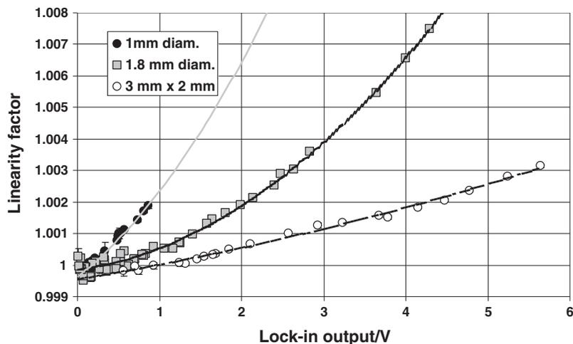
**Fig. 2.** Linearity factor of the “sprayed” MWCNT-coated pyroelectric detector as a function of the lock-in amplifier output for the three different spot sizes illuminating the active area of the detector. Also shown are the best quadratic fits to the data.
