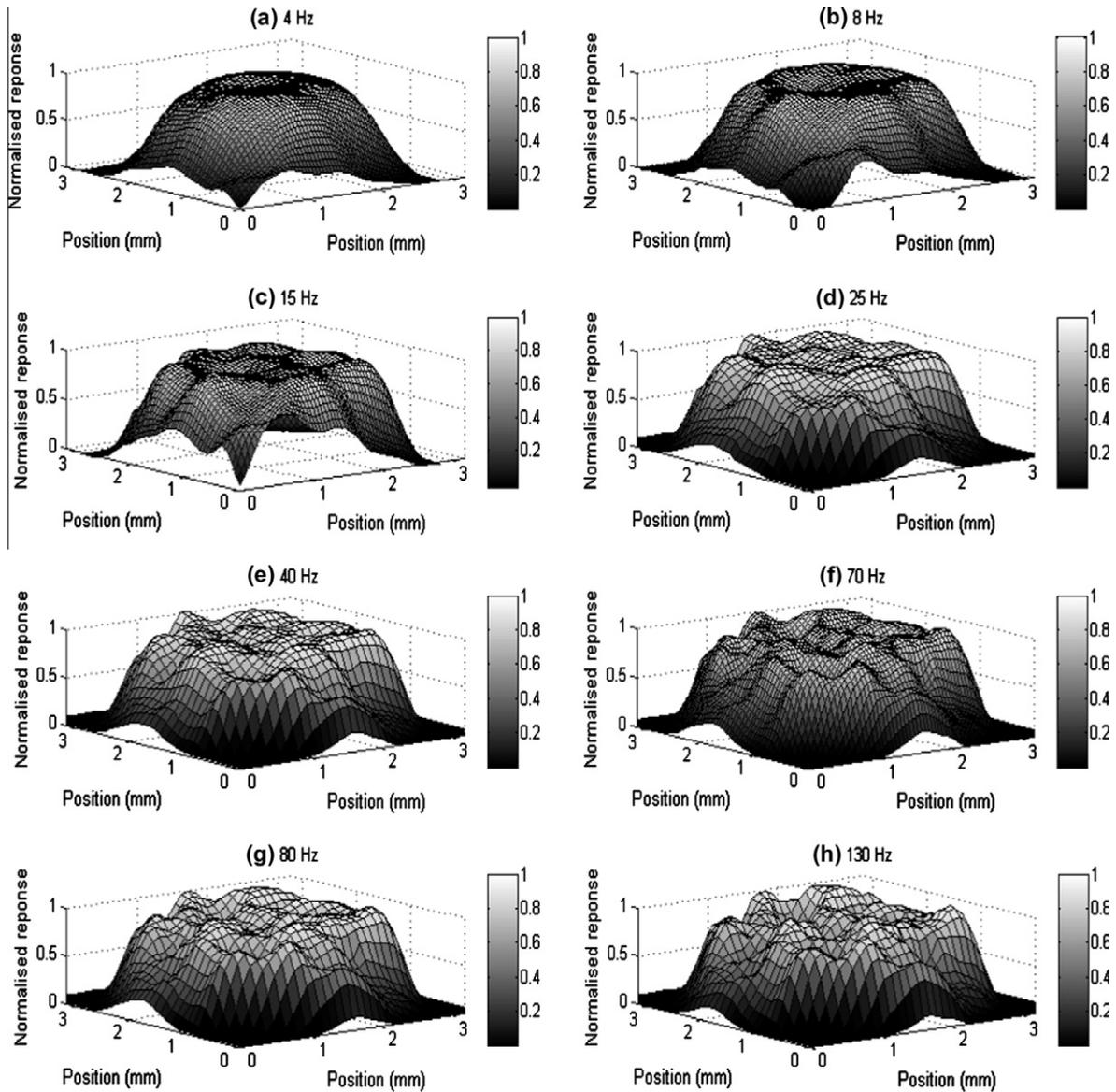
Fig. 4. Spatial uniformity of response of the “sprayed” MWCNT pyroelectric detector at eight different modulating frequencies in the 4 Hz–130 Hz range.
