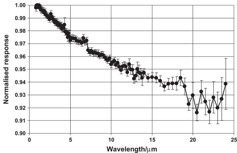
**Fig. 1.** Relative spectral responsivity of the “sprayed” MWCNT-coated pyroelectric detector normalised at 1.0  $\mu\text{m}$ . Error bars represent the  $1\sigma$  uncertainty of the measurements.
