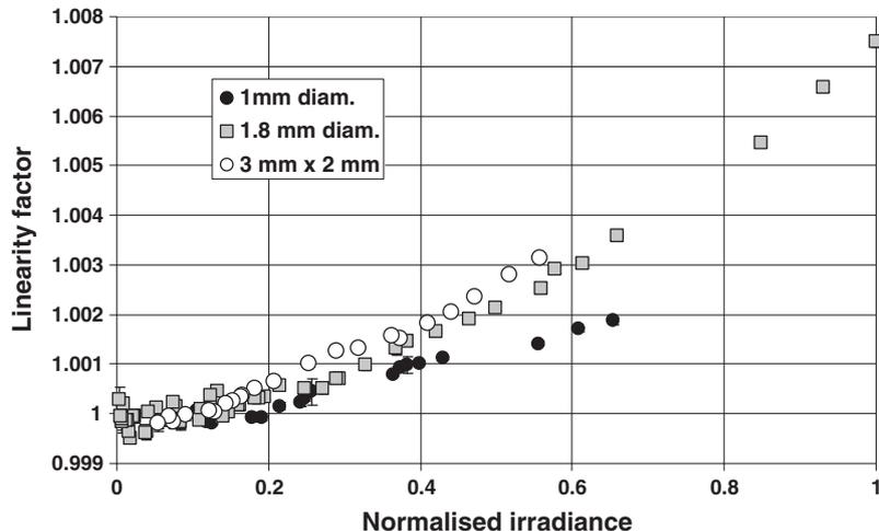
**Fig. 3.** Linearity factor of the pyroelectric detector coated with “sprayed” MWCNTs as a function of normalised irradiance for three different spot sizes illuminating the active area of the detector.
