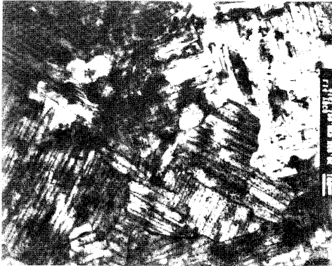
Figure 1: Transmission electron micrograph plan view of a 45° grain boundary. The straight, parallel lines running within grains are twin boundaries and indicate the orientation of the grain. The black irregularly curved line (most evident running left to right in the lower part of the picture) is the boundary between regions rotated 45° with respect to each other.
