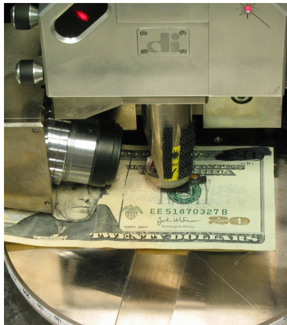
Figure 2. Dimension 3100 AFM at ASM, showing the scanner and a large test specimen.
