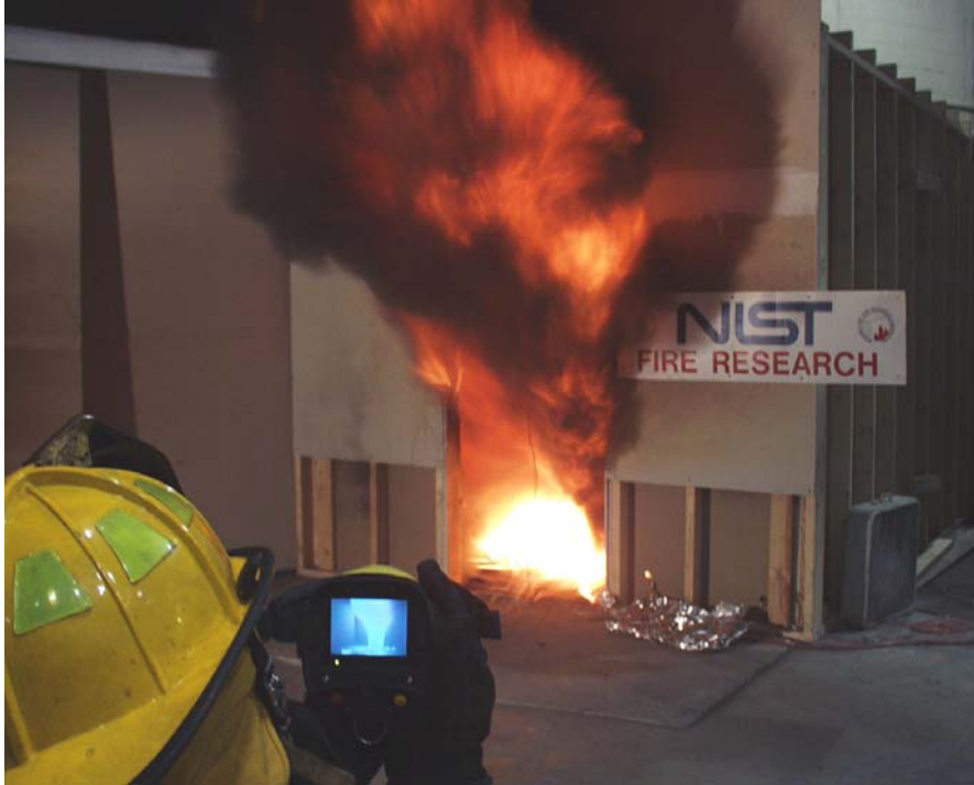
Figure 3.2 Testing the operational range of a thermal imaging camera.
