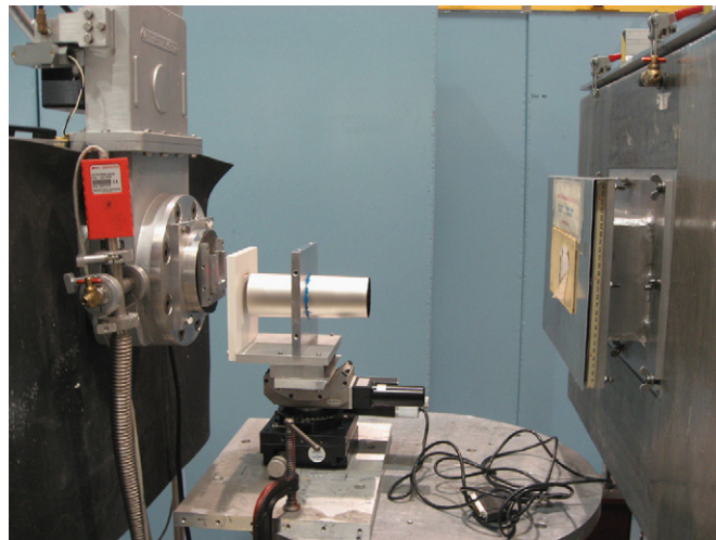
Fig. 6. The test mirror mounted on rotational and translation stages and installed on the NG7 beam line. At the left is the beam exit gate, and at the right is the SANS instrument box attached to the detector system. An annular aperture in the boron nitride plate placed before the optic defines the incident beam.
