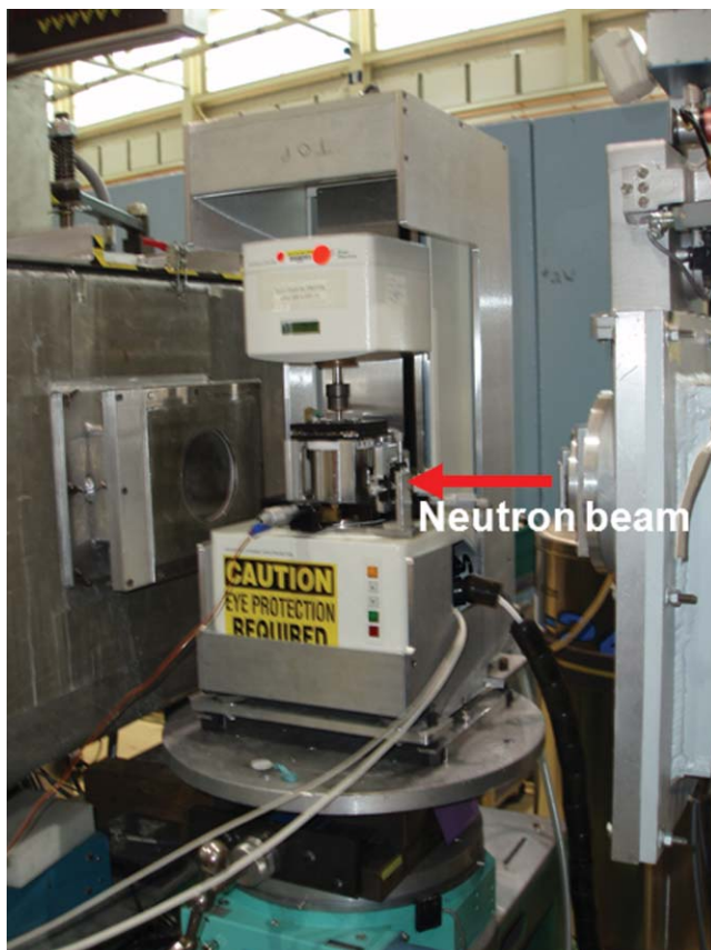
FIG. 2. (Color online) Rheometer installed on the NG3 SANS beam line at the NCNR. The arrow indicates the neutron path.
