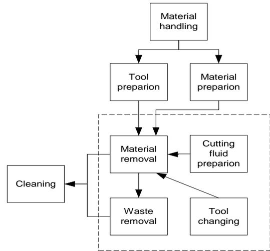
Figure 2. Machining system boundaries diagram
