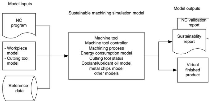
Figure 3. Proposed virtual machining model with environmental impacts analysis
