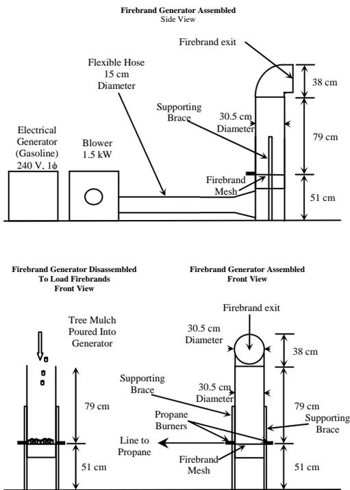
Figure 1 Schematic of NIST Firebrand Generator.
