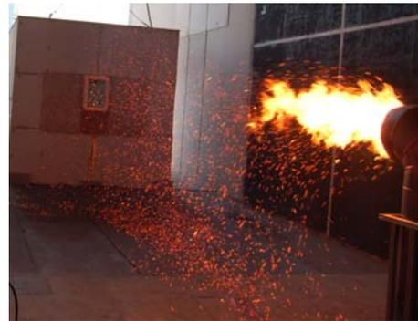
Figure 5 Typical experiment using NIST Firebrand Generator at BRI’s FRWTF. The mesh installed in this experiment was 20 x 20 (1.04 mm), the wind tunnel speed was 7 m/s, and the Firebrand Generator was located 7.5 m from the structure.
