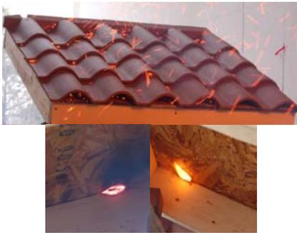
Figure 4 Images of experiments conducted using OSB/CT without bird stops installed. Intense SI was observed within the OSB base layer and eventually FI was observed. The wind tunnel speed was 7 m/s and the Firebrand Generator was located 2.0 m from the CT roofing assembly.
