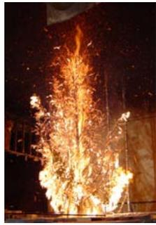
Figure 3 Photograph of a burning Douglas-Fir tree (5.2 m) used for firebrand collection.
