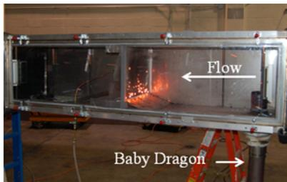
Figure 7 Picture of typical experiment using the Dragon's LAIR. A 14 x 14 (1.55 mm) mesh was being used when this photograph was taken.
