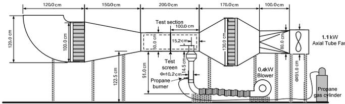
Figure 6 Schematic of Dragon's LAIR Facility. The Baby Dragon (coupled to 0.4 kW blower) as well as the firebrand seeding locating into the wind tunnel are shown.
