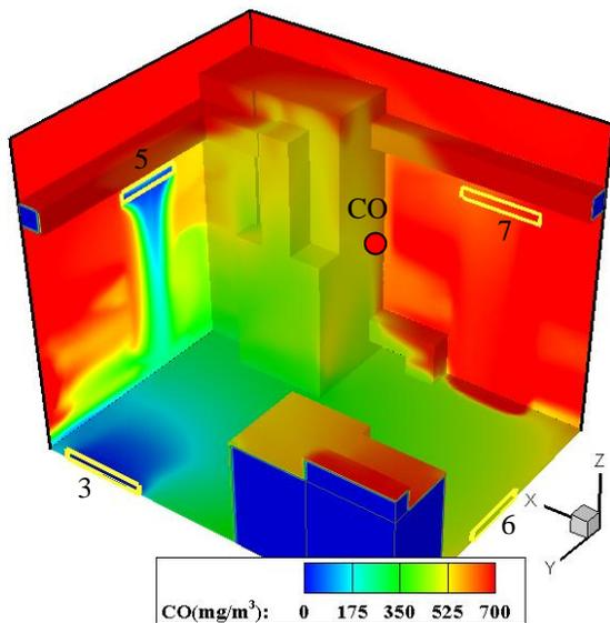
Figure 7 Distribution of CO concentration (mg/m<sup>3</sup>) in the utility room at end of the two hour simulation time
